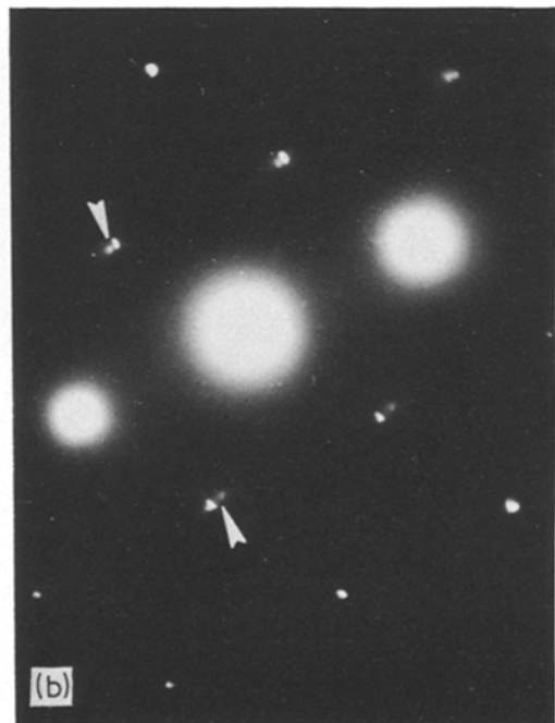
Figure 12 Cu-2.1% Ti-5% Al alloy, aged 120 h at 400° C. (a) BF (b) Associated SAD. [1 1 0] Z.A. Note the split (1 1 1) spots due to the loss of cubic symmetry.
