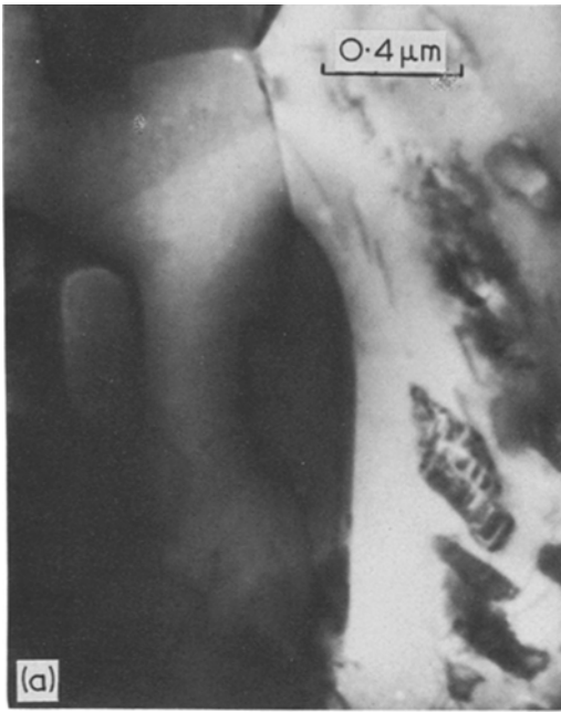
Figure 13 Cu-4% Ti alloy, aged at 700° C, 30 min. (a) BF. Shows incoherent equilibrium precipitates at the grain boundaries. (b) BF. Shows a PFZ near the grain boundary towards the continuous precipitates in one of the grains. Also shows discontinuous precipitates in other grain.
