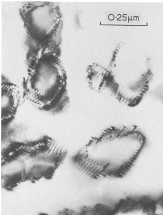
Figure 7 Cu-4% Ti alloy, aged at 700°C for 30 min Moiré fringes in contrast.
