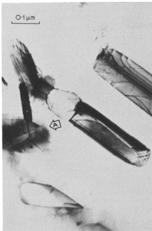
Figure 17 Cu-2.1% Ti-2.4% Al alloy, aged 1 h at 650° C BF. Observe the absence of discontinuous precipitation. Observe the internal structure of precipitates, probably due to faulted character.
