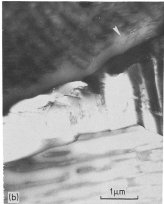
Figure 13 Cu-4% Ti alloy, aged at 700° C, 30 min. (a) BF. Shows incoherent equilibrium precipitates at the grain boundaries. (b) BF. Shows a PFZ near the grain boundary towards the continuous precipitates in one of the grains. Also shows discontinuous precipitates in other grain.
